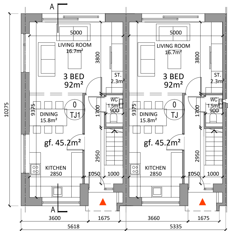
House Type TJ & TJ1 - Ground Floor Plan scale 1:100
